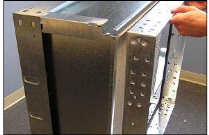
Figure 126: Positioning of the Prefilter Frame
