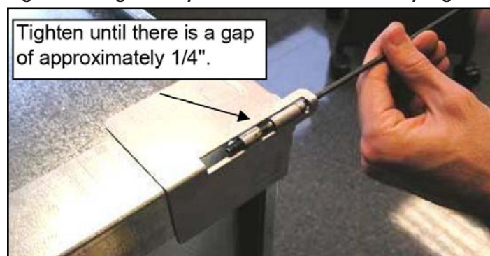
Figure 123: Tighten Cap Screw to 1/4 in. of the Coupling
